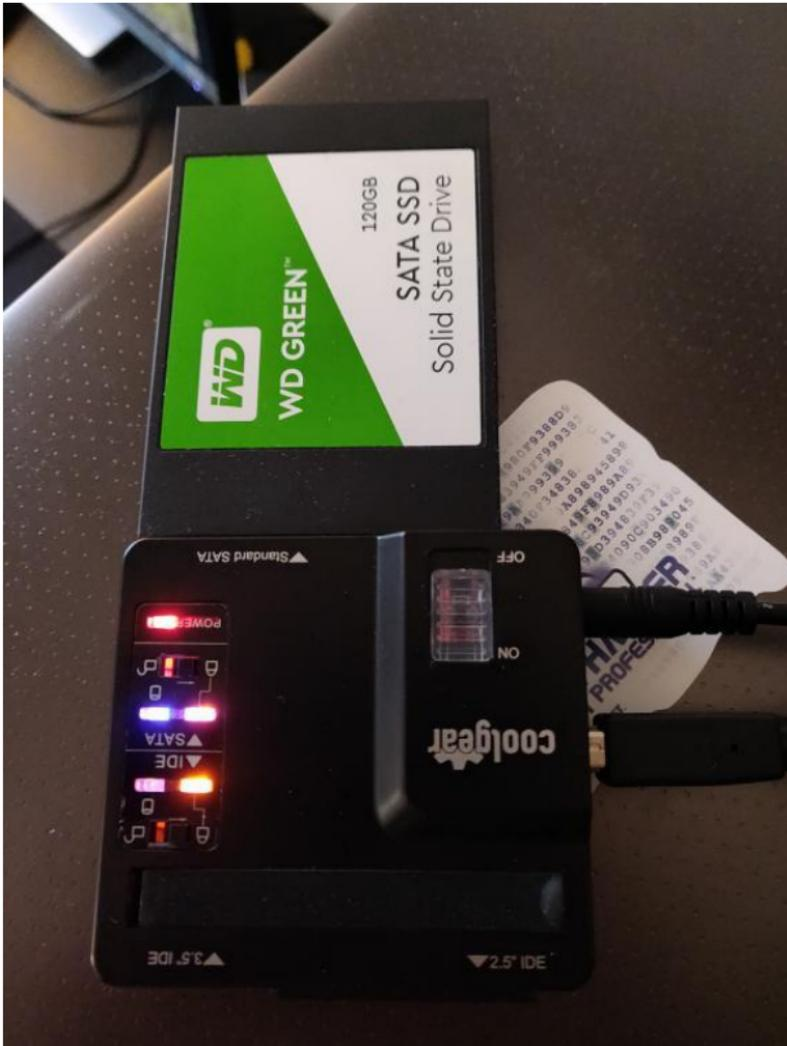
6 *Coolgear is the slightly discount version of a write protector. It works fine and is cheap (and unfortunately discontinued)*
